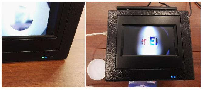
9. Run ElvaX software and make measurement. When the X-ray tube is turned on, the object indicator changes color to red.
