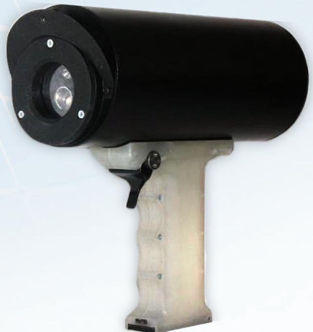
Instant on-site elemental analysis is one of the necessities of the modern mining industry. ElvaX Geo offers you accurate data and ease of operation during geo exploration or quality assurance. The instrument is designed specifically for long non-stop convenient operation. The unique 800 mm<sup>2</sup> analytical spot analysis increases averaging of inhomogeneous samples.
