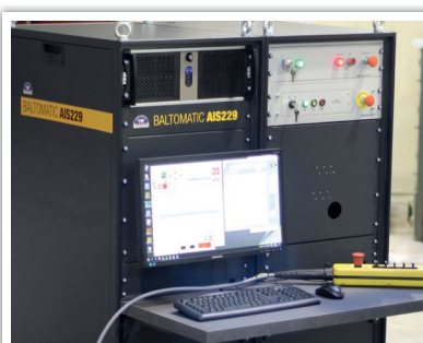
Control desk with PC rack 19" & LS1C2 control unit
