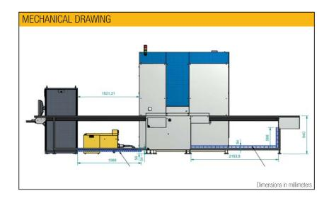
Composed of a shielded cabinet, a manipulator, conveyors In & out, an x-ray generator and tubehead from 160kV to 225kV, a flat panel & much more, the AIS500 is the answer to any business who wants to inspection their components from their production line at any stages of the manufacturing.
