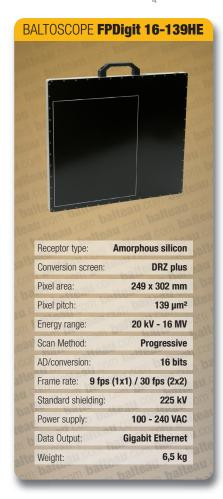
The FPDigit 16-139HE is high dynamic range x-ray detector. With a 16 Bit conversion and 139 μm² pixel pitch, this flat panel will offer a frame rates up to 30 frames per second (2 x 2). The acqusition of image will be made by Gigabit Ethernet communication. The FPDigit has internal shielding up to 225kV; Electronics being outside of the detector active area, an additional external shielding of the electronics can be added for use above 225kV
