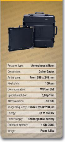
The Mobi-X is a portable flat panel detector. Thanks to its battery and Wi-Fi interface, a digital inspection can now be done anywhere. Moreover the Mobi-X is very light, robust and ergonomic which makes it easy to be used in harsh environment and conditions. Equipped with an internal memory, the Mobi-X can to store images in order to allow the operator to unload them later.
