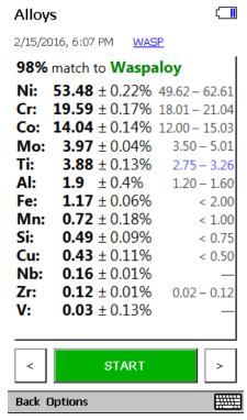
Figure 2. Testing screen of "Compare to alloy" mode.
