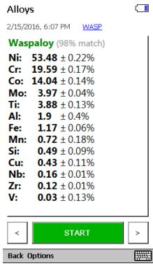
Figure 1. Testing screen of "Grade ID" mode.
