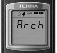
Figure 5 – LCD of the dosimeter (start of the submode of measurement result saving in the nonvolatile memory)
