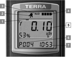
Figure 30 – LCD of the dosimeter (measurement results viewing)
