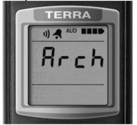
Figure 16 – LCD of the dosimeter (start of the submode of measurement result saving in the nonvolatile memory)
