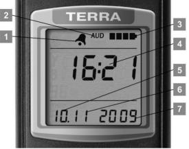
Figure 21 – LCD of the dosimeter (the clock mode)
