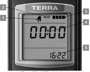
Figure 25 – LCD of the dosimeter (the alarm clock mode)
