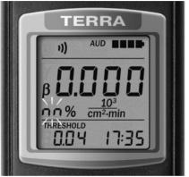
Figure 17 – LCD of the dosimeter (measurement restart)
