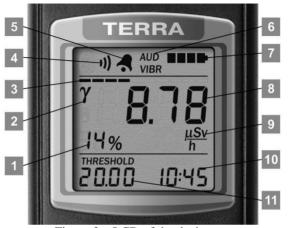
$\label{eq:Figure 3-LCD} Figure \ 3-LCD \ of the \ dosimeter \\ (the mode of photon-ionizing radiation DER \ measurement)$
