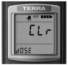
Figure 13 – LCD of the dosimeter (the sumbode of DE and DE accumulation time values resetting)
