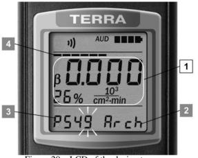
Figure 20 – LCD of the dosimeter (the submode of measurement result saving of surface beta-particles flux density)
