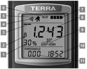
Figure 14 – LCD of the dosimeter (the mode of surface beta-particles flux density measurement)
