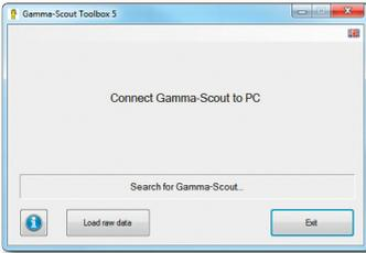
2. Connect the GAMMA-SCOUT® to the computer using the USB cable supplied. The data transfer process begins automatically and progress is indicated by a bar.
