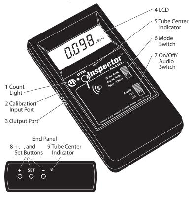
Whenever the IMI Inspector Alert is operating, the red count light (1) flahses each time a count (an ionizing event) is detected.
