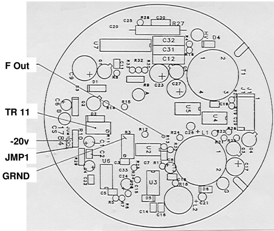
**Electrometer Board - Component Location**
