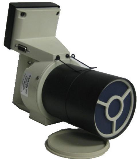
**RAM ION Open Window for Measuring Beta Radiation**
