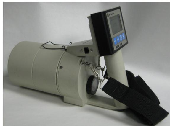
**RAM-ION shown with Tissue Equivalent Barrel (1000mg/cm<sup>2</sup>)**
