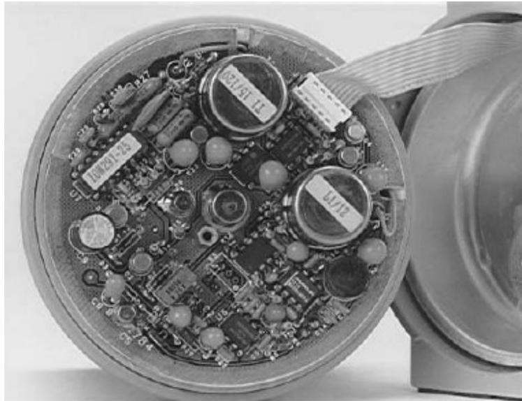
**Electrometer Board – Component Side**
