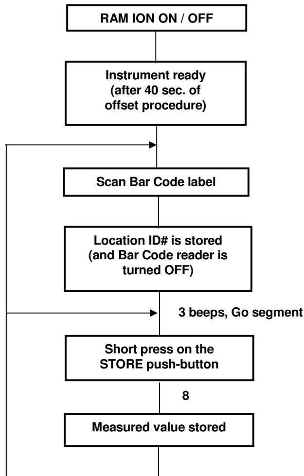
**Laser Scanner Operating Procedure**
