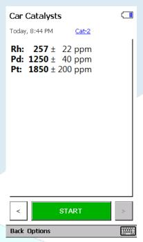
Figure 1. Measurement screen in Car catalyst testing mode.
