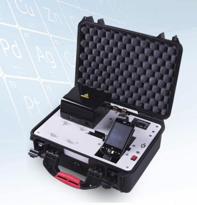
ElvaX Mobile is a portable EDXRF analyzer for testing a wide variety of materials.
