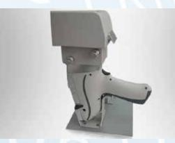
Use a laboratory stand to prevent X-Ray scattering when analyzing small objects or light matrix samples.
